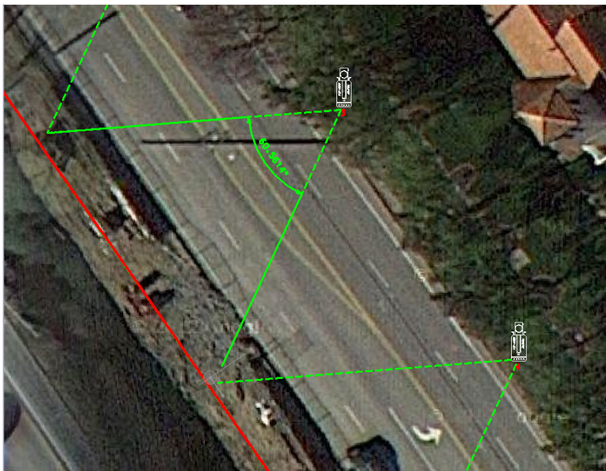
Figure 37: Top View Scanner Position-Wall Alignment (TopoDOT™)
