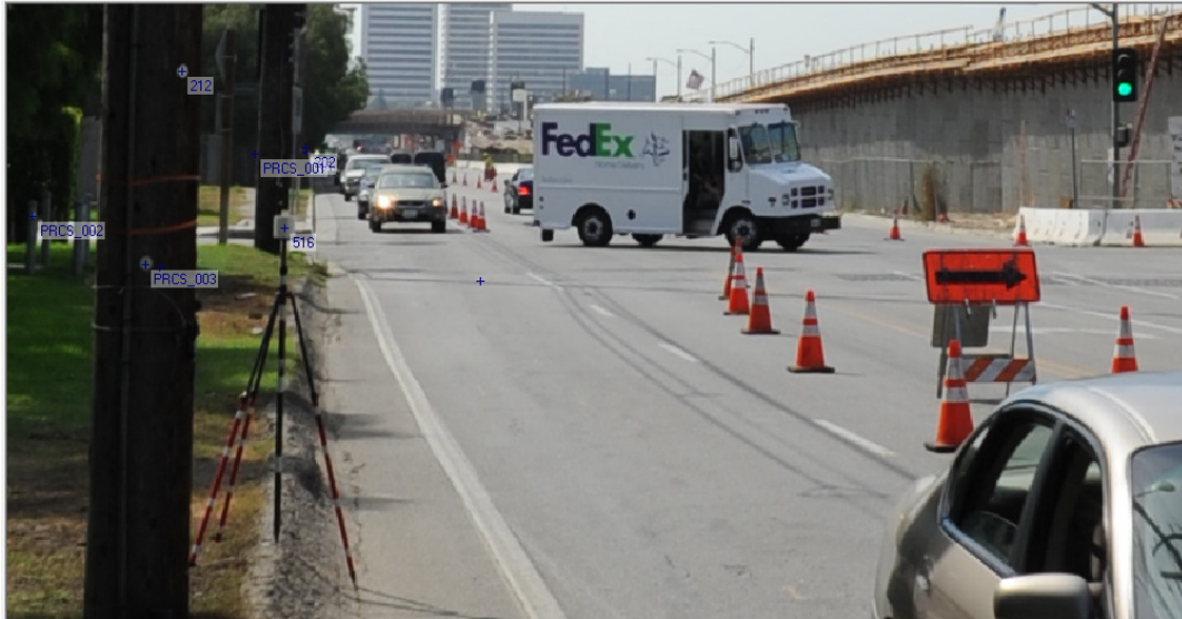
Figure 6: Reference targets along roadside
